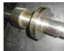
Pinion shaft wear
